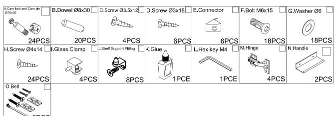
STEP 1: Place a small amount of glue on each Dowel(B) and insert into the Side Panel(C2a,C2b) and Bottom Panel(C6).Use a Phillips Head Screwdriver to insert the Cam Pin(A) to the Side Panel(C2a,C2b) and Bottom Panel(C6) and Top Panel(C1).
